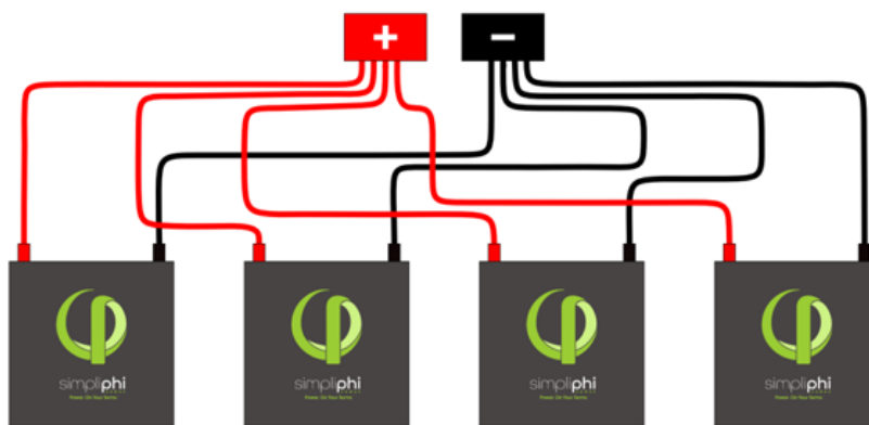
Figure 9.0 - Four PHI Batteries in Parallel
